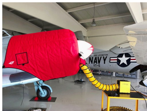
Yak 11 Insulated Engine Cover
