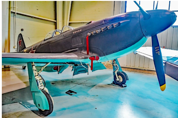
Yakovlev Yak 3 Oil Cooler Inlet Plugs (In Wing Root), Belly Scoop Plug
