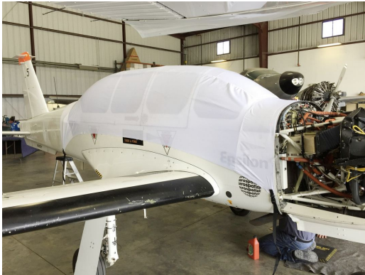
Socata TB30 Epsilon Canopy Cover, test fit cover
