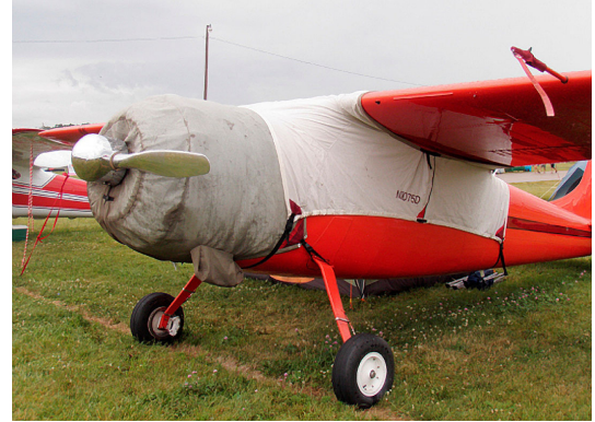
Cessna 195 Over-Top Canopy Cover & Engine Cover
