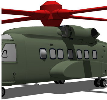
Sikorsky S-92 Main Rotor Hub Cover
