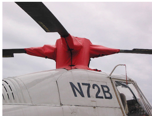
Sikorsky S58 Rotor Hub Cover
