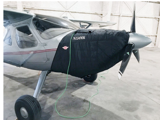
Glasair Aviation Glastar, Sportsman 2+2 Insulated Engine Cover
