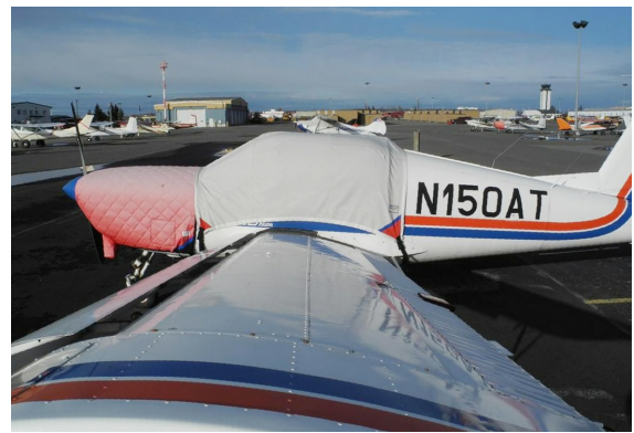
Koliber 150A Canopy Cover, Insulated Engine Cover
