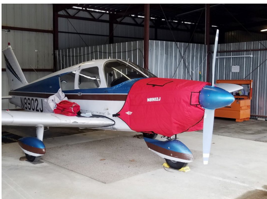
Piper PA-28-180 Insulated Engine Cover with Oil Filler Preheater Access and Inlet Preheater Access Ports Flaps
