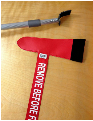
Piper Aerostar Pitot Cover and Installation Tool
