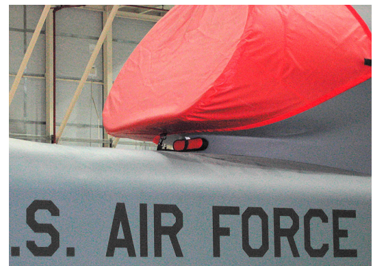
Intake Cover with small inlet plug
