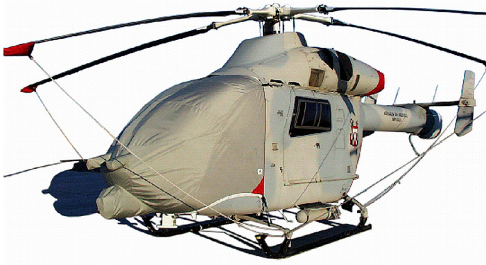
MD900 Forward Bubble Cover (w/Radome), Blade Tie-Downs
