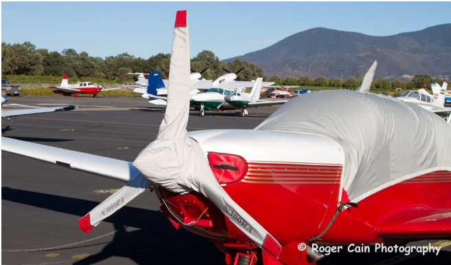
Mooney M20M Bravo 3-Blade Prop Cover, Engine Plugs ENGINE PLUGS PREVENT BIRD NEST FOD. Piper Saratoga Engine Cowling Bird's Nest
