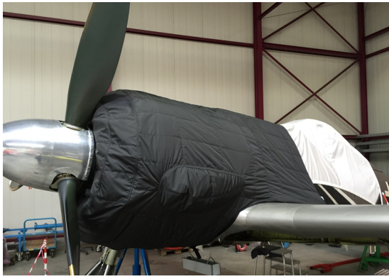
Focke Wulf 190 Canopy Cover & Insulated Engine Cover
