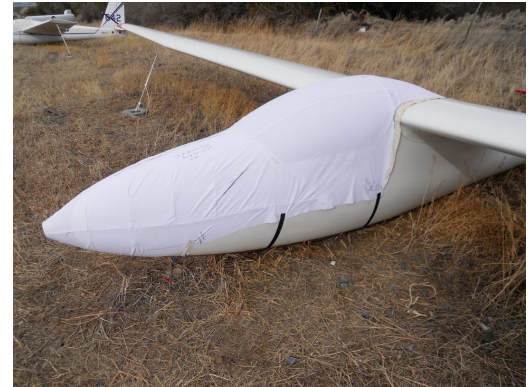
Laister LP-49 Canopy/Nose Cover, test fit cover
