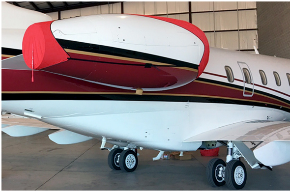
Intake/Exhaust Covers, 3-Strap Type. Successfully installed by two crew, one ladder.
