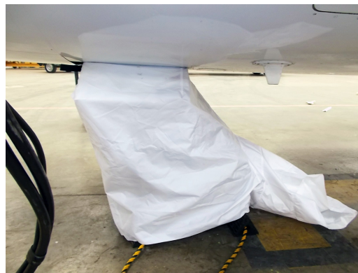
Q400, Nose gear landing/tire covers - Cold Weather Ops
