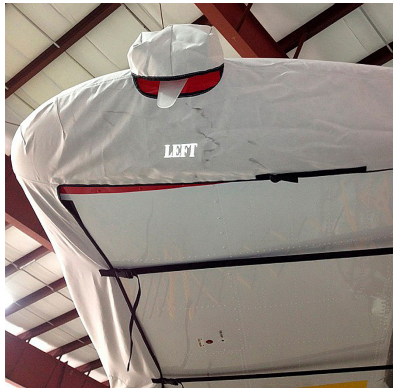
De Havilland Twin Otter Wing Cover wing tip detail
