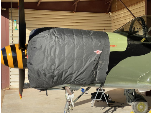
Nanchang CJ6 Insulated Engine Cover
