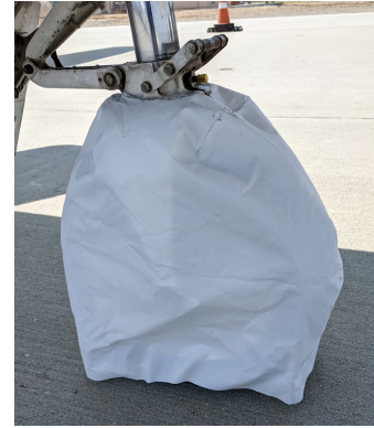
CJ1 Nose Gear Tire Cover, test fit
