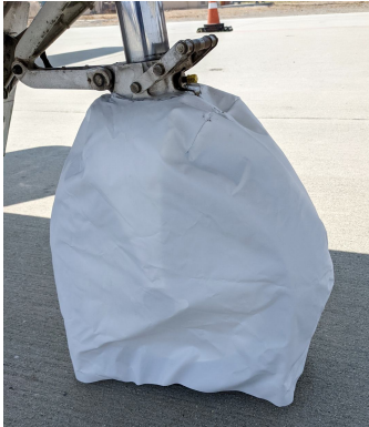
CJ1 Nose Gear Tire Cover, test fit
