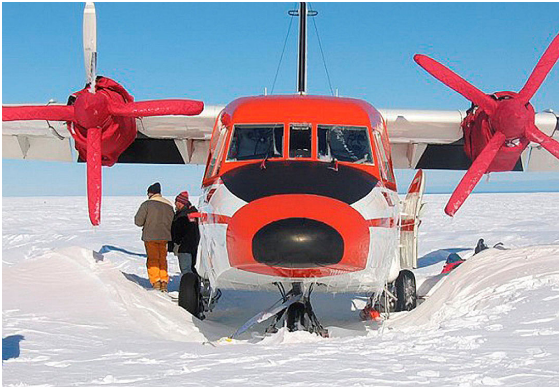
Casa 212 Insulated Engine & Propellor/Spinner Covers Prop Tie-Down, Various Models (secures with a hook to engine nacelle)
