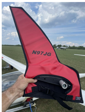
Schempp-Hirth Ventus-2B winglet/wingtip pads
