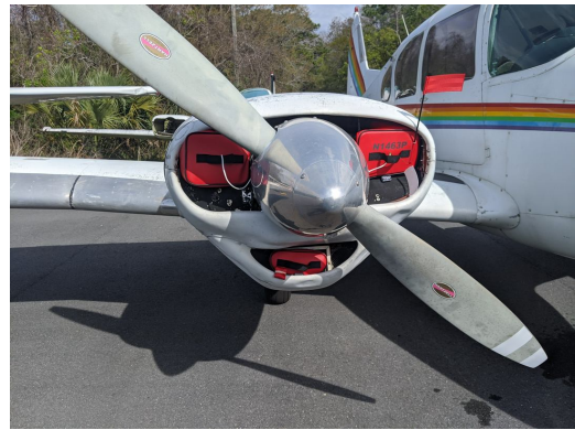
Piper PA-23 Apache Engine Inlet Plugs (fit needs improvement)
