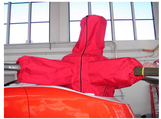
MH-65C Engine Area Cover, Swash Plate Aperture, Rotor Hub cover set, P/N: A365-210 MH-65C Rotor Hub Cover w/ OADS Tube Cover detail
