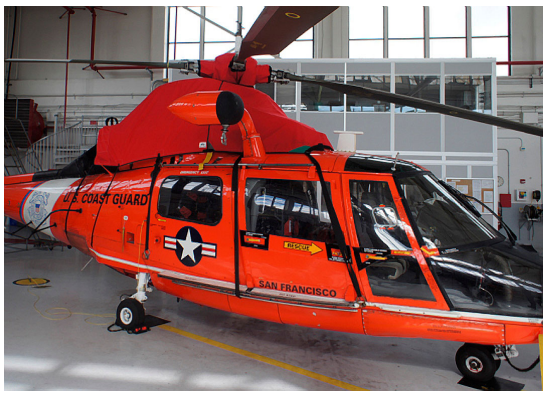
MH-65C Engine Area Cover, Swash Plate Aperture, Rotor Hub cover set, P/N: A365-210 MH-65C Rotor Hub Cover w/ OADS Tube Cover detail
