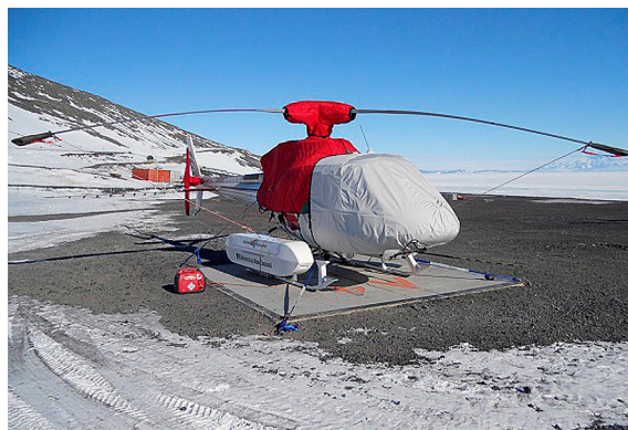
AS355 Bubble Cover w/ Cargo Mirror, Blade Tie-downs, Insulated Engine, Insulated Main Rotor Hub & Insulated Tail Rotor Covers
