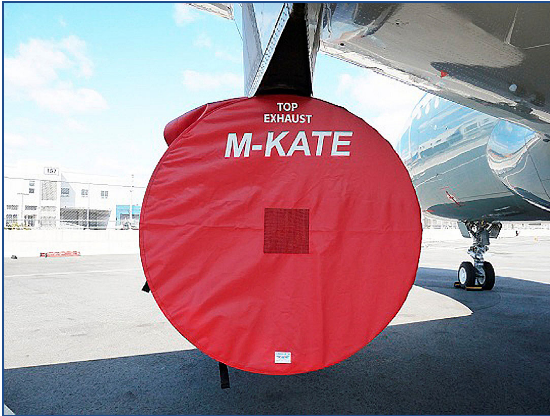
Airbus A319 Intake/Exhaust Covers set, IAE V2500
