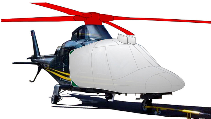
Agusta 109 Bubble, Rotor Hub & Blade Covers (illustration)
