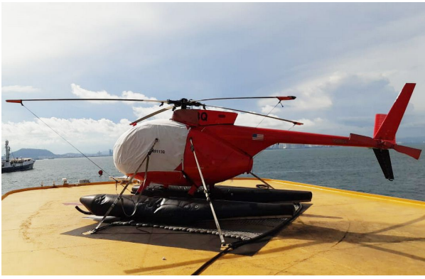
Hughes 500C (369HS) Bubble Cover, Blade Tie-Downs
