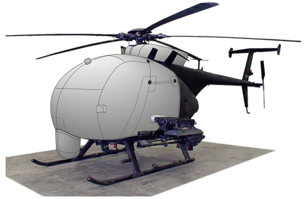
MH-6J Bubble, Flir & Doghouse Covers (illustration)
