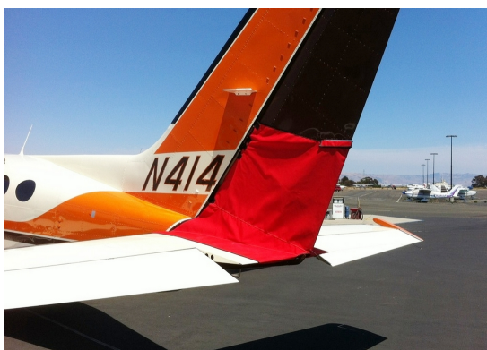
Cessna 414 Rudder Openings Cover (bird barrier)
