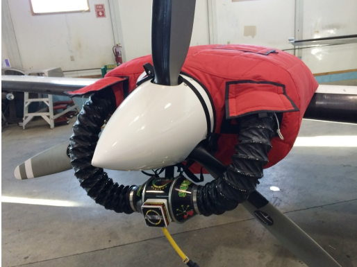
Cessna 402 Insulated Engine Cover with Heater
