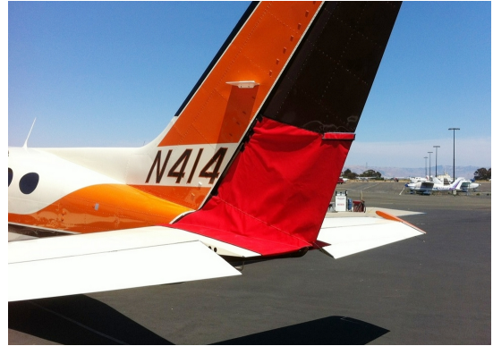
Cessna 414 Rudder Openings Cover (bird barrier)
