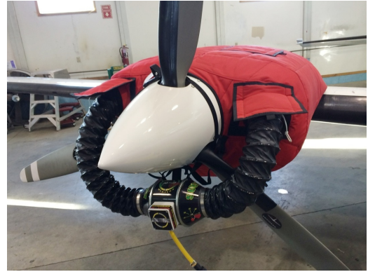
Cessna 402 Insulated Engine Cover with Heater
