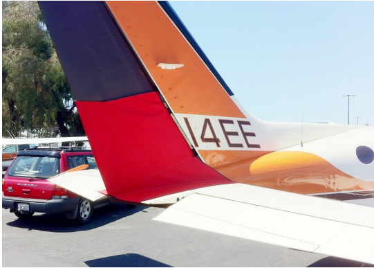
Cessna 414 Rudder Openings Cover (bird barrier)
