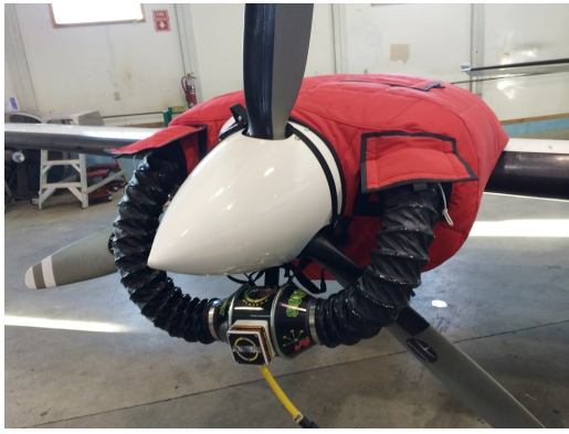
Cessna 402 Insulated Engine Cover with Heater
