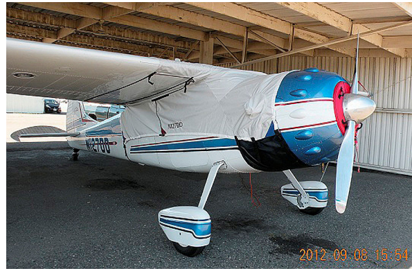
Cessna 195 Over-top Canopy Cover, 24" fwd ext to cover cowl ring gap, gas cap ext. & under belly cowl ring gap mesh covering
