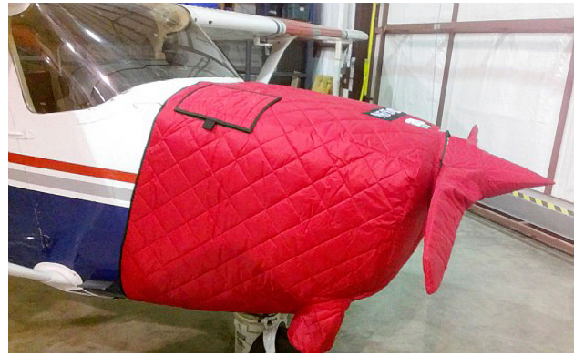
Cessna 172 Insulated Engine Cover w/ Oil Filler Door flap and Insulated Prop/Spinner Cover
